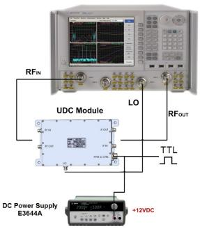
To cover all possible combinations, multiple calibrations are needed for both UP and Down converters. As mentioned before, to reduce the number of calibrations and measurements, consider how to group all the required measurements to minimize the calibration time.
