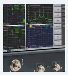
RF & Microwave converters are complex modules requiring specialized techniques for their measurement and characterization. In this tech brief we present three different examples of UP/Down converters and their different measurement strategies, looking for an accurate and efficient approach.
