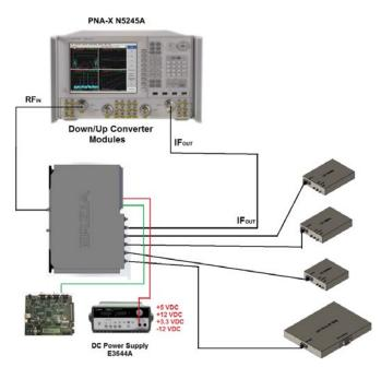
In this case, to measure P1dB, NF and S-parameters 26 channels are needed to cover all possible sub-bands for the down-converter. Due to the big number of channels, different calibrations were done for each type of measurement. In this case, due to the complexity, image signals or possible leakages were measured with the Signal Generator and Analyzer, by applying signals covering frequencies from 0.1 to 40 GHz for all the sub-bands.
